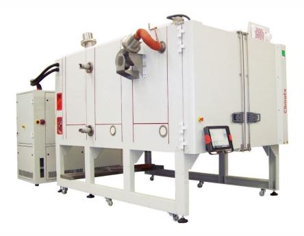
With a useful volume of 5,6m³, this environmental chamber has a monobloc steel structure and a temperature range from -70°C to +180°C. The particularity of this equipment is the height position of its test cabinet, allowing free access under the chamber to position means of customer testing.
