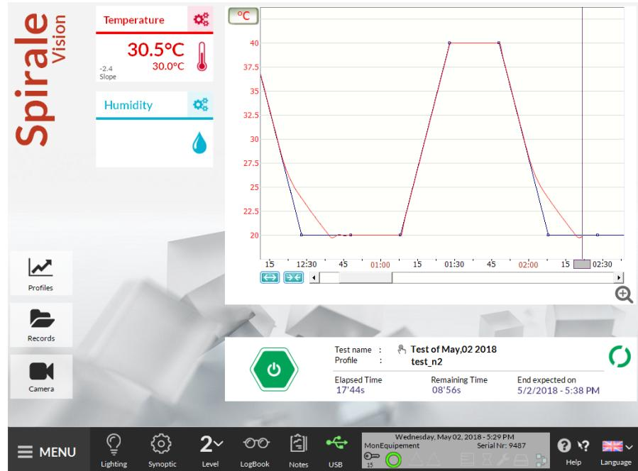
Laboratory mode : Freely select a programme and monitor it while running using the CycleWin recorder
