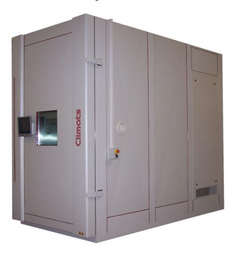
6 m³ one-piece Hot Cold Humid environmental chamber indented to receive several layers of product over a 2500 mm inside height.
