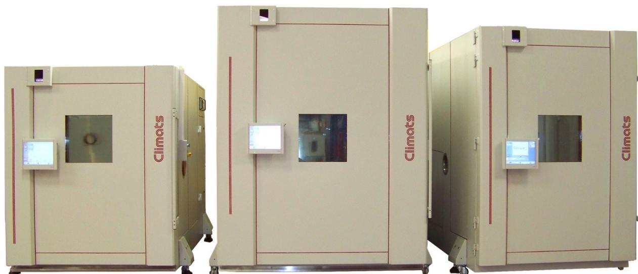
Manufacturing of 3 environmental chambers of 4, 6 and 8 m<sup>3</sup> meant for Export to carry out Photovoltaic (PV) Modules tests standards.
