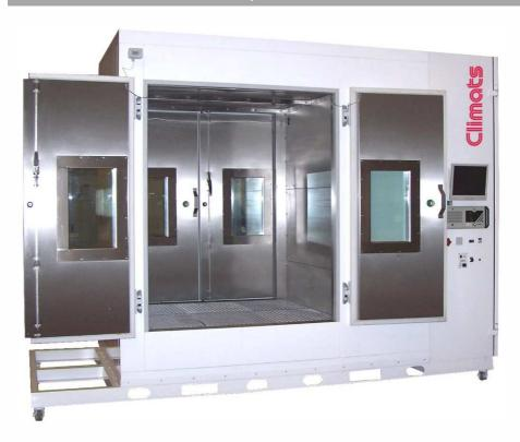
2700 dm<sup>3</sup> one-piece environmental chamber intended for tests in laminar flow atmosphere, within a temperature range from  $+20^{\circ}$ C to  $+60^{\circ}$ C, with air speed rates inside the volume between 0,3 and 0,5 m/s during plateau.
