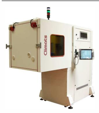
Taylor-made to perfectly contain a whole test bench, this climatic chamber will be crossed by a complex drive system enabling to test moving products in extreme conditions.
