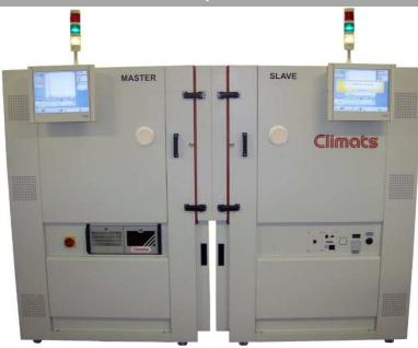
Joined but independent, these two chambers of Excal 140 "hot cold humid" type enable window panes or other materials to be tested under two different climatic conditions which could, eventually, stand for outside and inside atmospheres.
