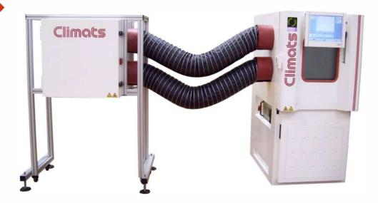
This chamber, from our standard range Excal (8 volumes from 140 to 1800 dm<sup>3</sup>), is transformed into an air generator supplying a recipient cabinet, also made by Climats.
