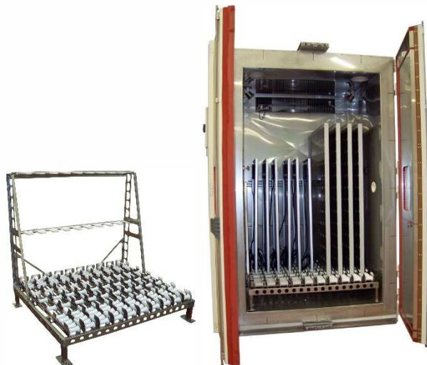
Rack to easily receive the photovoltaic panels
