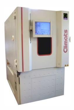
**Very compact and powerful environmental chamber** intended for Rapid Change of Temperature tests on electronic boards.
