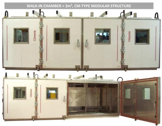
Two environmental chambers, at first totally independent in term of functioning, but that could be put together for tests on longer planes' wings.
