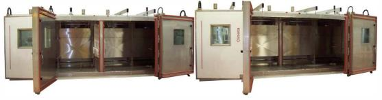
A supervisor connected to the two control PC enables to synchronize these two equipments in order to get a very good regulation within the temperature and humidity whole range.
