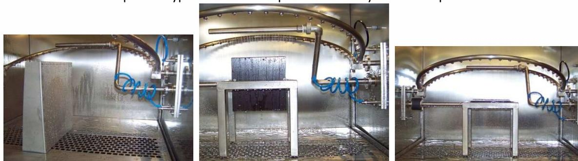
The water used for the sprinkling is recycled thanks to a retention tank. Fillings and drainings are automatic.
