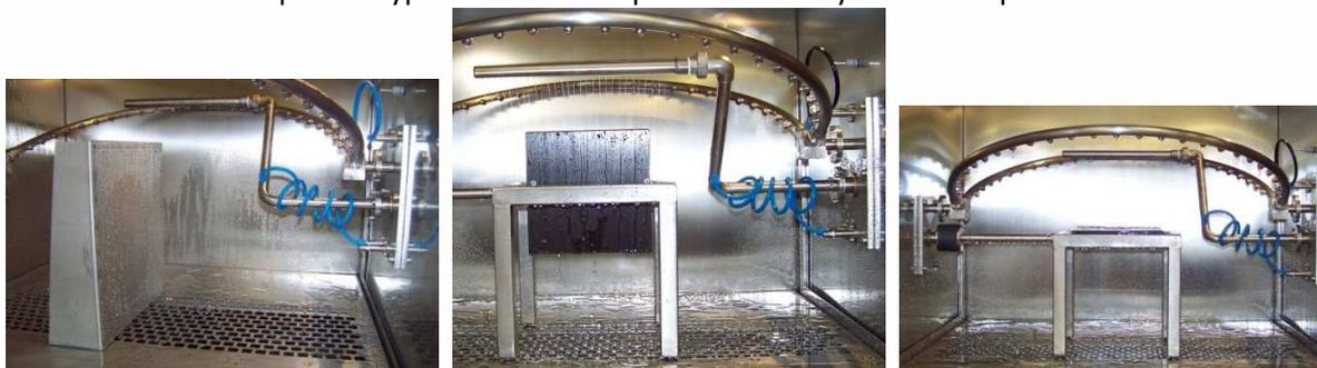
The water used for the sprinkling is recycled thanks to a retention tank. Fillings and drainings are automatic.
