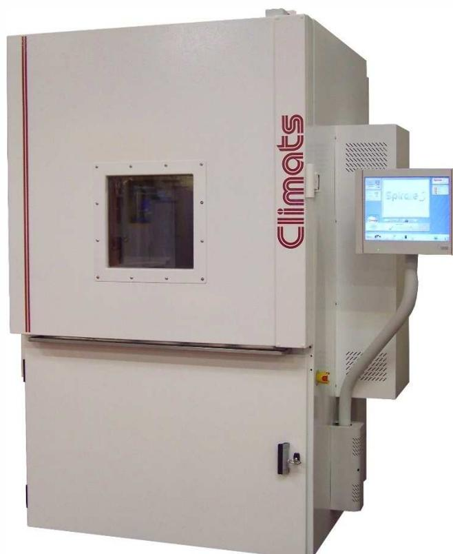
This chamber is made of a cabinet that includes 3 distinct devices, enabling watertightness tests according to procedures described in standards of the main automobile manufacturers.
