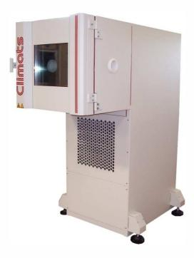
110 litres thermal chamber with an advancing cabinet under which an engine test bench can be positioned.
