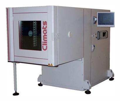
343 dm³ climatic chamber, <u>adaptable onto a shaker</u>, with plate accessories to be used as a standard chamber.
