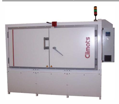
1350 dm<sup>3</sup> thermal chamber, meant for burn-in of 300 kg of components at positive temperature (70/85°C).
