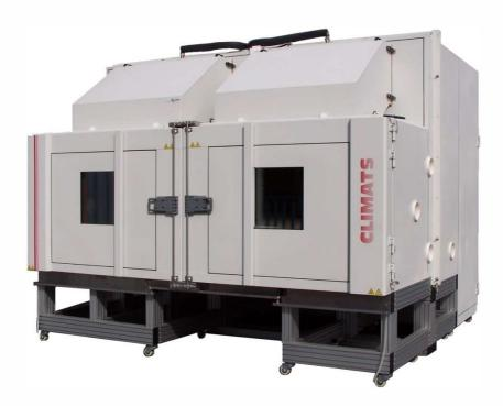
4000 dm<sup>3</sup> environmental chamber for vibration and temperature combined tests.
