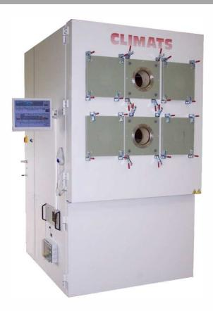
Very powerful air generator (closed circuit), equipped with 6 high / low temperature sheaths (inside  $\emptyset$  150mm, length 5m).
