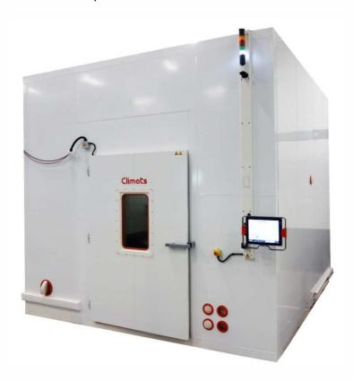
The choice of this equipment is characterized by the speed with which climatic conditions are set up in temperature and humidity, thus reducing the duration of the tests, but also ensuring a very good stability of the climatic parameters.
