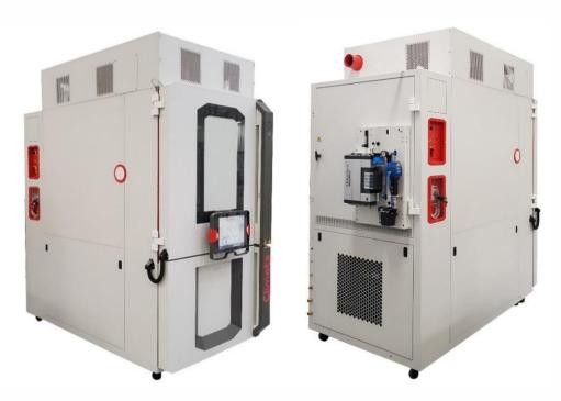
The special feature of this enclosure is that it achieves extreme temperatures, and perform thermal cycling, in the temperature range of -80°C to +265°C. In addition, this equipment can reach a speed cooling rate greater than 10°C/min linear from +200°C to -40°C, with a load of 10kg of electronic boards positioned on a shelf. As a reminder, the linear speed corresponds to the instantaneous speed of the machine unlike the average speed which defines a duration.
