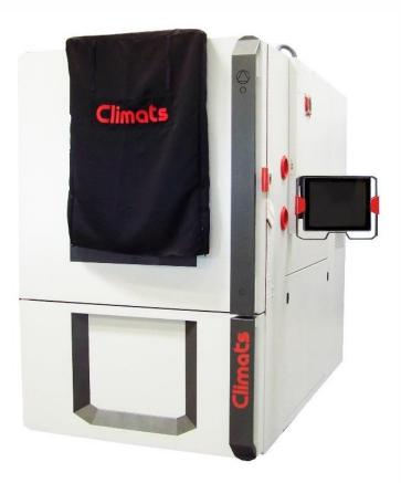
With a useful volume of 1000 liters, this chamber covers a **temperature range of -70°C to +150°C**, with a **cooling rate of +70°C to -55°C of 15°C/min** average(s) with 100 kg a load of aluminum and 1500 WHATTS of dissipation, and vice versa.
