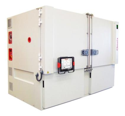
With a useful volume of 2000 dm³, this aging chamber covers a temperature range from  $+20^{\circ}$ C to  $+100^{\circ}$ C and reaches an average variation speed of around 1°C/min between  $+20^{\circ}$ C to  $+70^{\circ}$ C, with load of 50 kg of composite materials. The double door provides excellent ergonomics for flat loading large parts.
