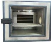
The **TM benchtop** consists of a stainless steel cabinet and of a removable griding on racks where the samples can be put onto.
