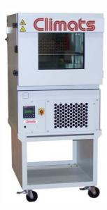
**Benchtops** enable a product to be put through temperature tests in order to reveal its possible defects or to determine its life length.
