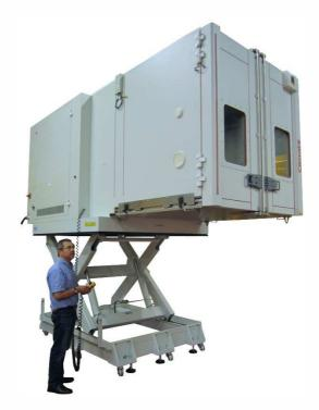
**Mobile on two axes and assisted for its vertical moves**, this hot – cold- humidity chamber enables to test wide products in vibration and temperature combined conditions.
