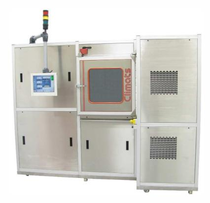
This one-piece chamber **meets the requirements of the MIL-STD-810F standard (Method 506.4)** which defines laboratory tests intended to certify materials of military use, as well as civilian, against environmental damages due to water.
