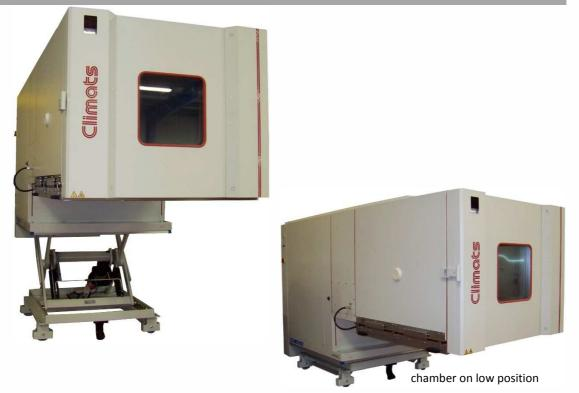
Set on two 5 m long rails perfectly aligned, this chamber – meant for electronics area – can still move on two axes in order to easily free the working space for the tests preparation.
