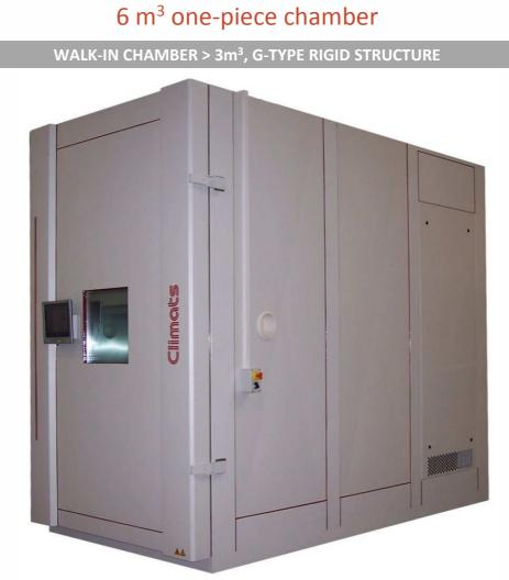
**6** m<sup>3</sup> **one-piece Hot Cold Humid environmental chamber** indented to receive several layers of product over a 2500 mm inside height.
