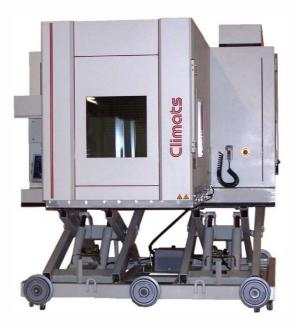
Hot-Cold-Humid Rapid Temperature Cycling type of climatic chamber (1200 dm³) set on a lifting table intended for combined temperature / vibrations tests.
