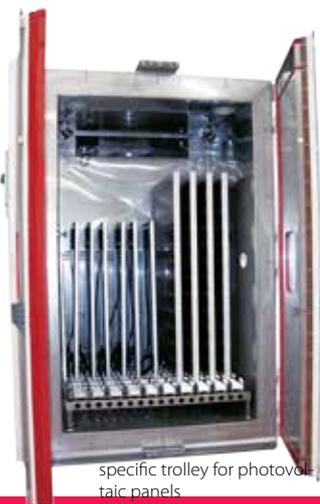
specific trolley for photovoltaic panels
